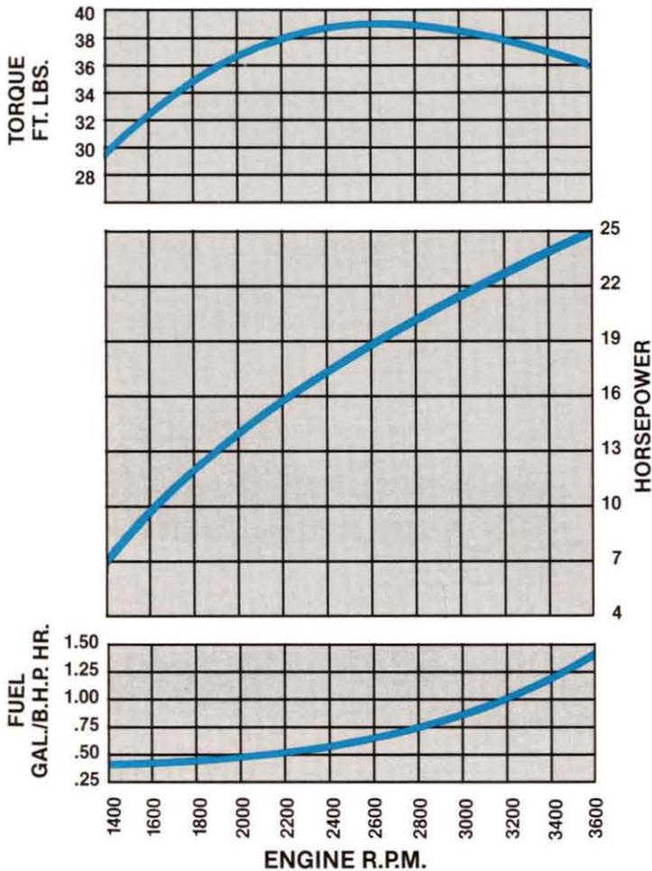
Note: Propeller load will decrease fuel consumption rate.
